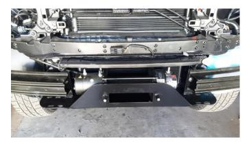
Use provided jig to locate where to cut fairlead hole:
