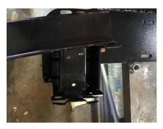
Wings and winch tray bolted to vehicle:
